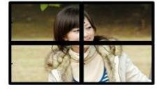
The physical gap of the LCD screen causes the complete image to be forcibly pulled apart for a certain distance, resulting in image deformation and distortion. Part of the image is lost by adjusting the size of horizontal splicing and vertical splicing, but the image is not deformed and distorted, as shown below:
