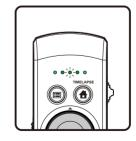
Green LED indicates charging mode. LED will be off when fully charged.
